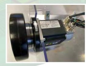
Mounted from outside the AGV, the bolts go through the motor mounting plate from the front and attach to the outside of the AGV body. This does not affect the clearance between the AGV motor wheel and the AGV body.
