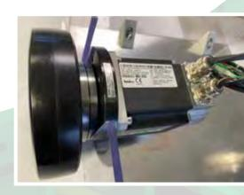
Mounted from inside the AGV, the bolts go through the motor mounting plate from the rear and attach to the inside of the AGV body. Take care in leaving enough clearance between the AGV motor wheel and the AGV body.
